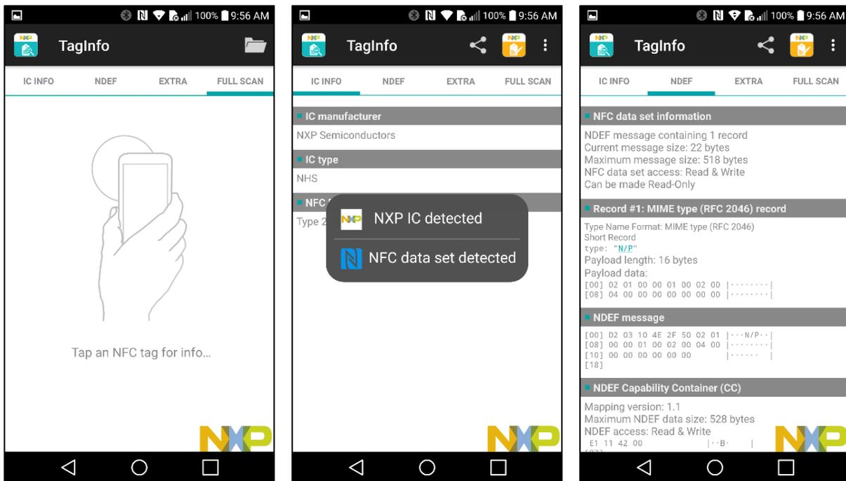
**Figure 8. Smart Phone Reading an Unprogrammed FleX-NFC FHE Starter System**
