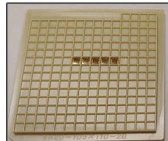
**Figure 9 - FleX-NFC Chips in waffle pack**
