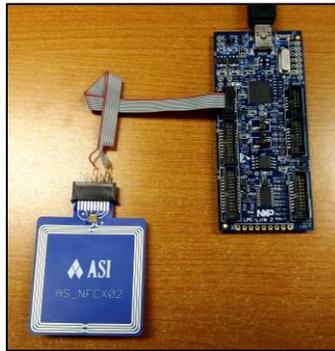
**Figure 4. Connecting the LPC-Link2 to the FleX-NFC FHE Starter System**
