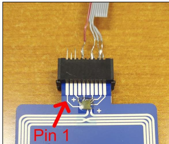
**Figure 5: FleX-NFC Programming Header**
