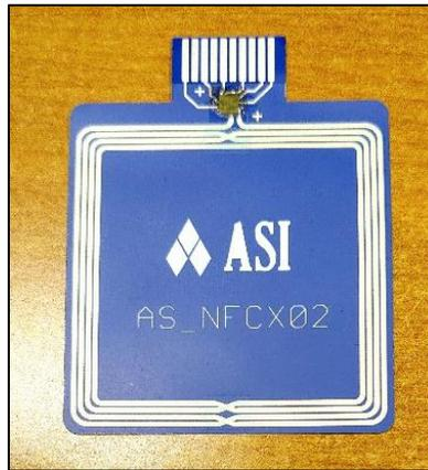
**Figure 1. FleX-NFC AS\_NHS3100P.fhs FHE Starter System**
