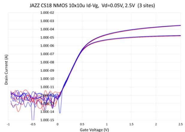
Figure 4: Jazz CS18 NMOS Transistor pre-FleX (red) and post-FleX (blue)
