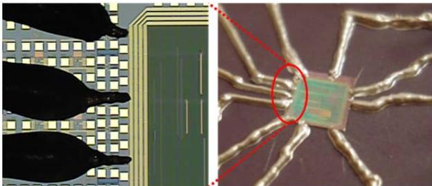
**Figure 7: Conformally Attached FleX IC Prototype with Direct Write Flexible Interconnects**
