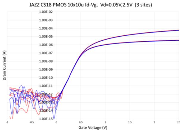
**Figure 5: Jazz CS18 PMOS Transistor pre-FleX (red) and post-FleX (blue)**
