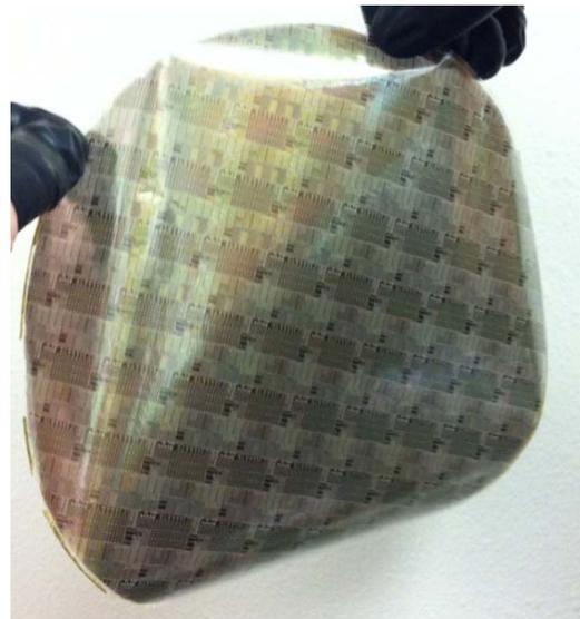
Figure 3: Jazz CS18 Wafer After FleX Processing
