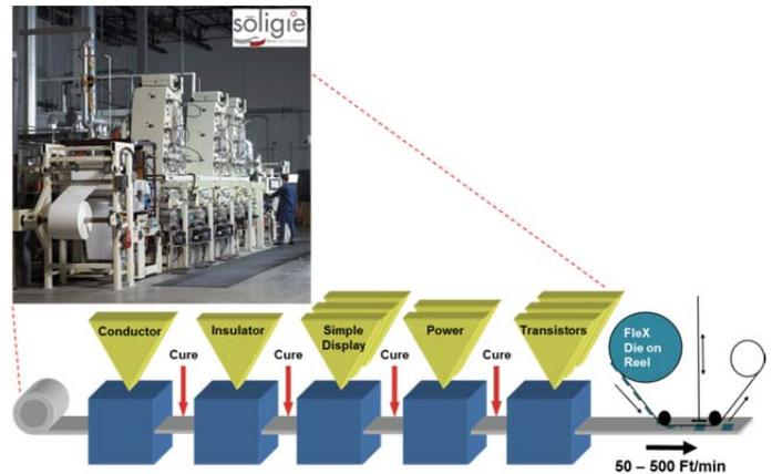
**Figure 8: Flexible Hybrid Manufacturing Line**
