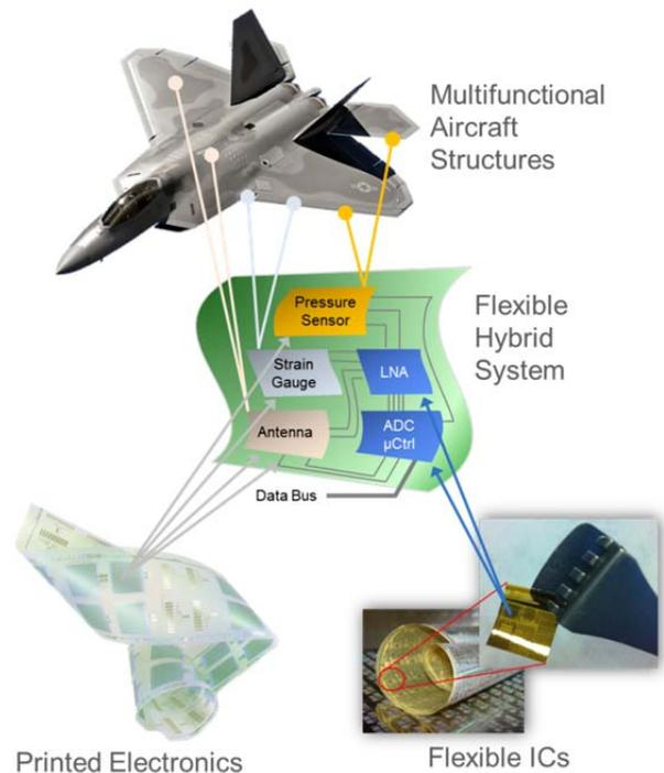
**Figure 6: Flexible Hybrid Systems Integrated into Multifunctional Aircraft Structures**
