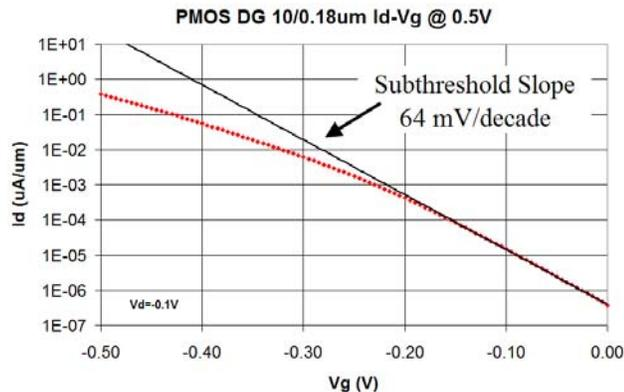
**Figure 3.** Flexfet ULP near-ideal subthreshold slope
