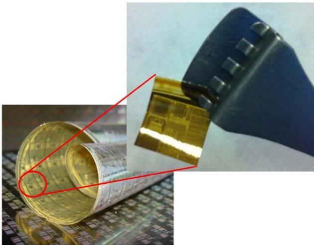
**Figure 2.** A transparent die and 200mm FleX wafer built on 3 metal Aluminum Flexfet CMOS.
