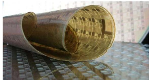
**Figure 1.** FleX Silicon On Polymer Wafer.
