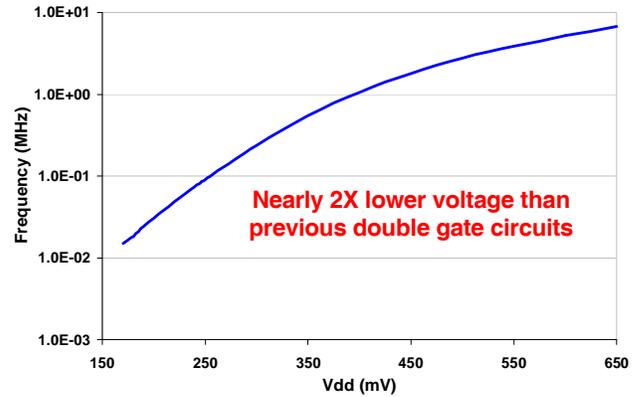
**Figure 8.** Flexfet 130nm MUGFET ring oscillators operating down to 170mV
