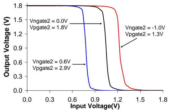
**Figure 5.** Flexfet 180nm MIGFET Dynamic Threshold Control - experimental data at 1.8V showing bottom gate voltage control of an inverter
