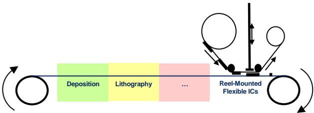
**Figure 3.** FleX “chips” added to Roll-to-Roll processing lines.
