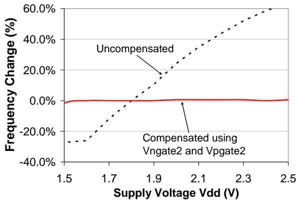
**Figure 7.** Flexfet 180nm MIGFET Dynamic Threshold Control - experimental data at 1.8V showing supply voltage compensation of a ring oscillator
