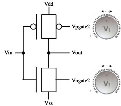
**Figure 4.** Flexfet MIGFET inverter showing Dynamic Threshold Control
