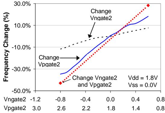
**Figure 6.** Flexfet 180nm MIGFET Dynamic Threshold Control - experimental data at 1.8V showing frequency tuning of a ring oscillator
