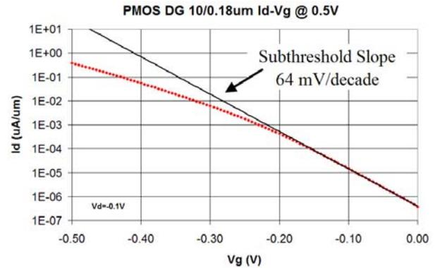
**Figure 9.** Double Gate (MUGFET) Flexfet PMOS FET with near-ideal subthreshold slope
