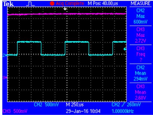
Fig. 11: Complete Interconnect Failure Signal
