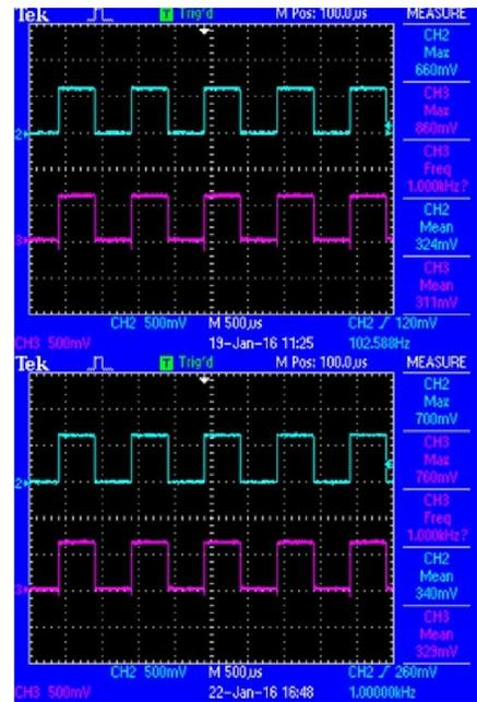
Fig. 9: Pre (top) and Post (bottom) Test I/O Waveforms
