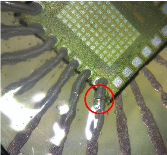
Fig. 12: Crack in Printed Interconnects on VDD Line
