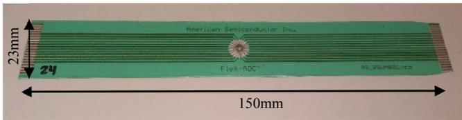
Fig. 4: Rainbow FHE Test Vehicle
