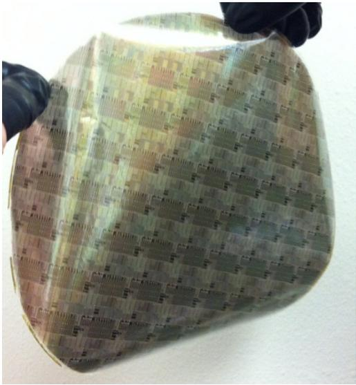
Figure 5: Jazz CMOS Wafer After FleX Processing
